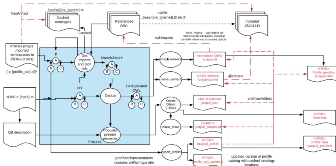
**Figure 12:** Profilewiz experimental tool for identifying overlaps between semantic models and generating minimal schemas
