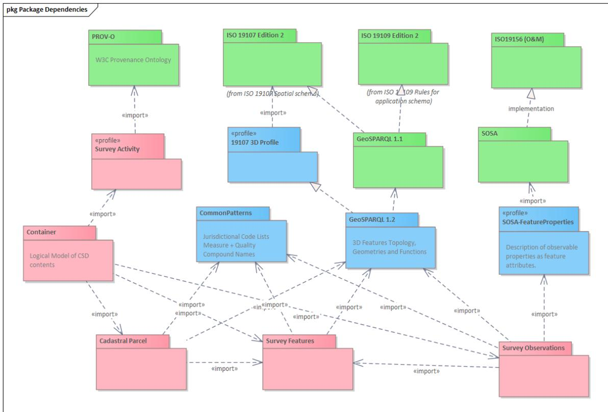
**Figure 7:** Package Modules of the 3DCSM and applied standards
