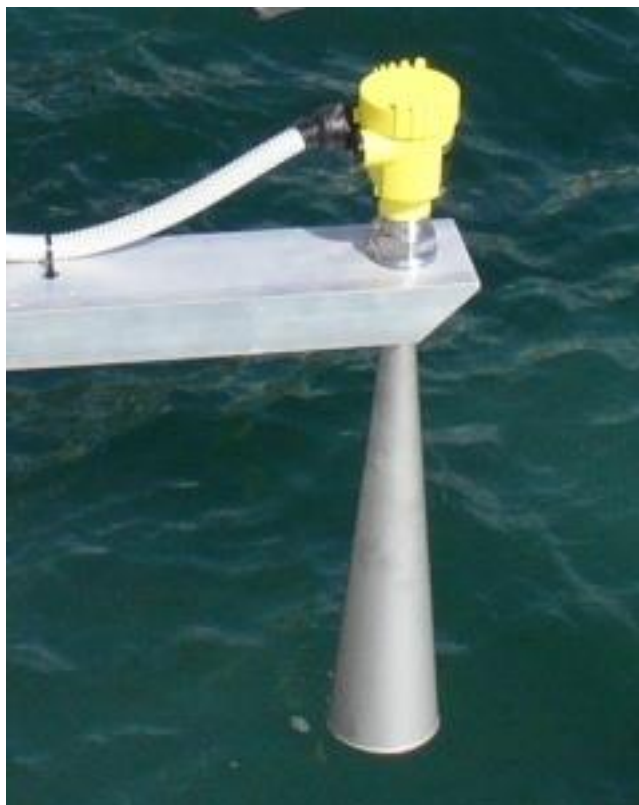
Figure 4 - Typical Microwave radar sensor used at many Australian Ports. This particular unit is a Vega Pulse 63 on a wharf in Gladstone harbour.
