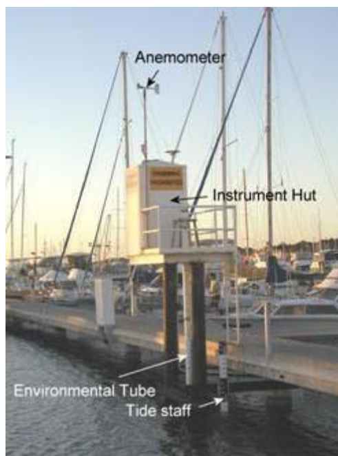
Figure 5 - Tide gauge at Hillarys, Western Australia.
