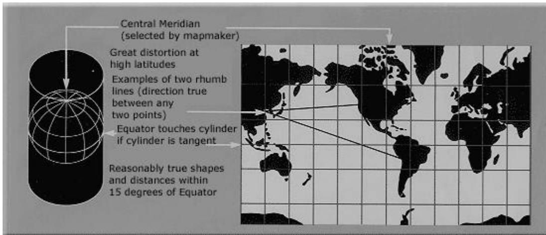
**Used** for navigation or maps of equatorial regions. Any straight line on the map is a **rhumb line** (line of constant direction). **Directions** along a rhumb line are true between *any* two points on map, but a rhumb line is usually *not* the shortest distance between points. (Sometimes used with Gnomonic map on which any straight line is on a great circle and shows shortest path between two points).
