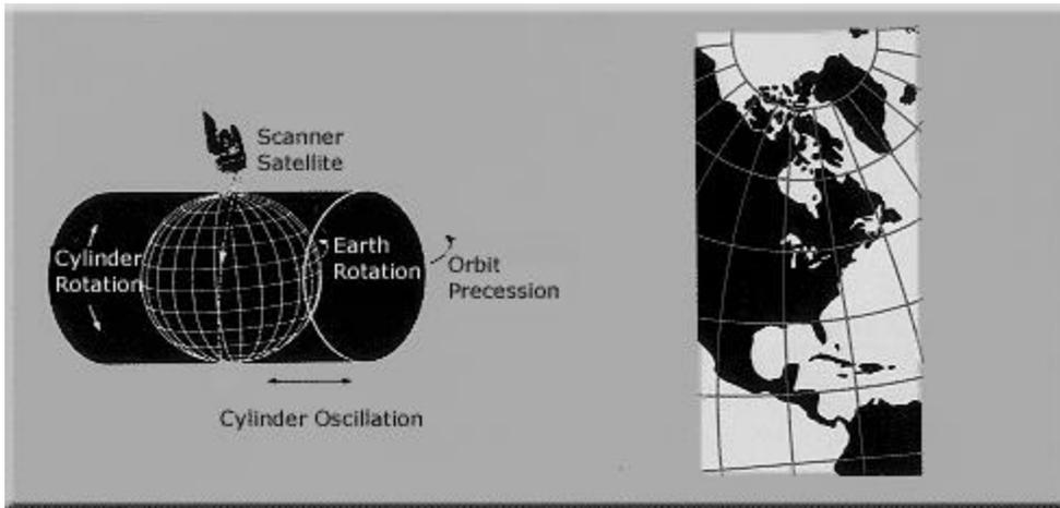
This new space-age conformal projection was developed by the USGS for **use in Landsat images** because there is no distortion along the curved groundtrack under the satellite. Such a projection is needed for the continuous mapping of satellite images, but it is useful only for a relatively narrow band along the groundtrack.
